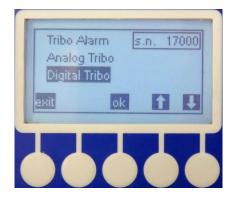
If using a digital probe with RS485 connection, in the first 10 seconds after the switch on, the control unit interrogates the probe and waits for the response signals for establishing the communication, the screen flashes the indication that the probe is not present.
