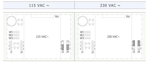
In 24 Vac and 24 Vdc powered versions, the J3 and J4 jumpers are not used.
