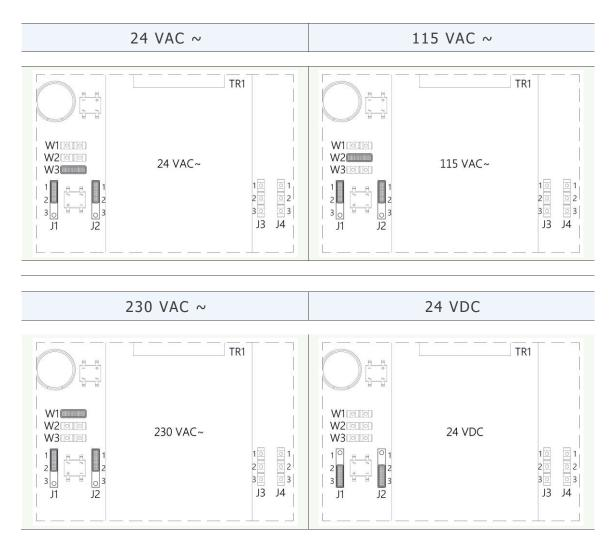
In the versions powered at 24Vac and 24Vdc the output voltages cannot be 115Vac or 230Vac.
