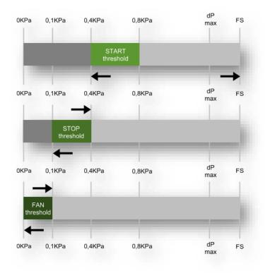
These values contribute to the execution of the functions relative to the automatic cleaning and post-cleaning cycles.
