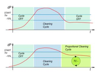
If, at the end of valve activation, the pressure differential drops by over 15% with respect to the "dP Start Cleaning" value, the cycle is suspended to resume when this value is exceeded again.
