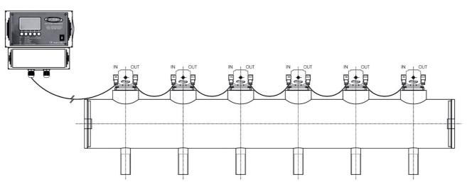
connect the other electro valves sequentially using the wiring harness with the PG7 connectors respecting the IN -> OUT polarity, assemble the gaskets to ensure the IP seal of the circuit.
