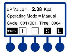
The displayed information is: the operating mode, the internal dust filter pressure, active outputs and the time necessary to activate the next output.
