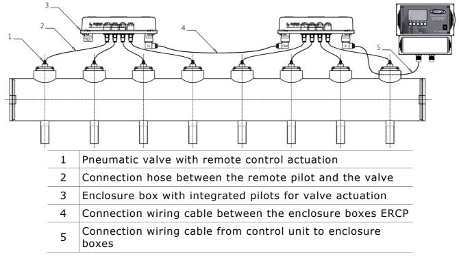
Connect the ERCP enclosure boxes in sequence using the wiring harnesses with the DIN 43650 connectors to be fixed to the cylindrical sideburns.
