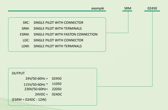
The code SRM02450 represents a single pilot with terminals (SRM) powered by a 24 V 50 Hz voltage (02450).
