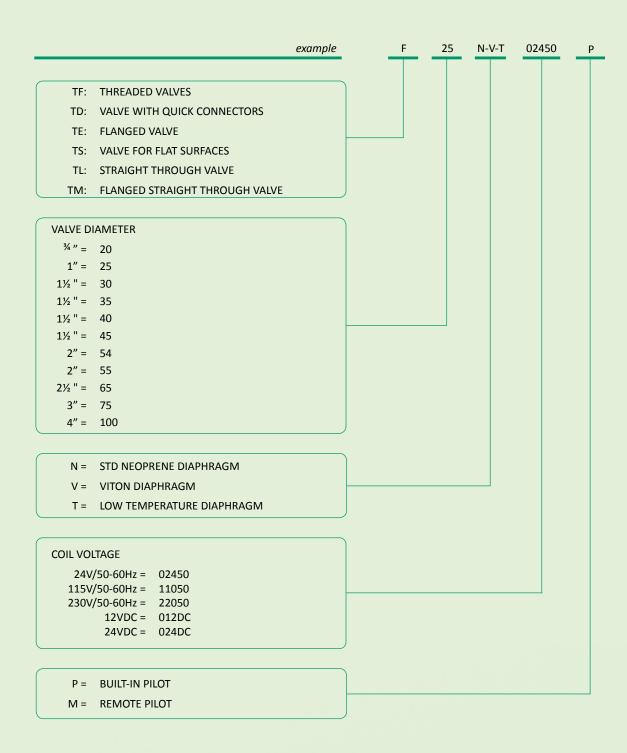
The Code TF025NPB represents a threaded valve of the TF series, which has an electric pilot installed (P), a 1" diameter (25) and is powered by a 24V 50Hz voltage (02450).
